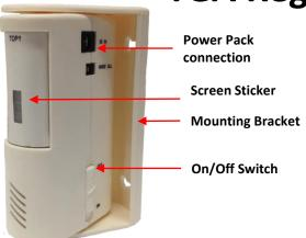
The PIR Motion Sensor detects movement with its narrow curtain beam. When a resident crosses the beam's path, the staff will be alerted through their nurse call system. The PIR Kit includes a custom cable with a 6.3mm mono straight plug and a 3 meter lead to be used for connection to the nurse call system. It is powered by a 9V Power Pack or a 9V Battery.
