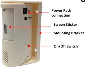
The PIR Motion Sensor detects movement with its narrow curtain beam. When a resident crosses the beam's path, the staff will be alerted through their nurse call system. It has an exclusive RF Transmitter that communicates with our Wireless Receiver (RRU) or Call Point with a receiver module. It is easy to install and program, and is powered by a 9V Power Pack or a 9V Battery.
